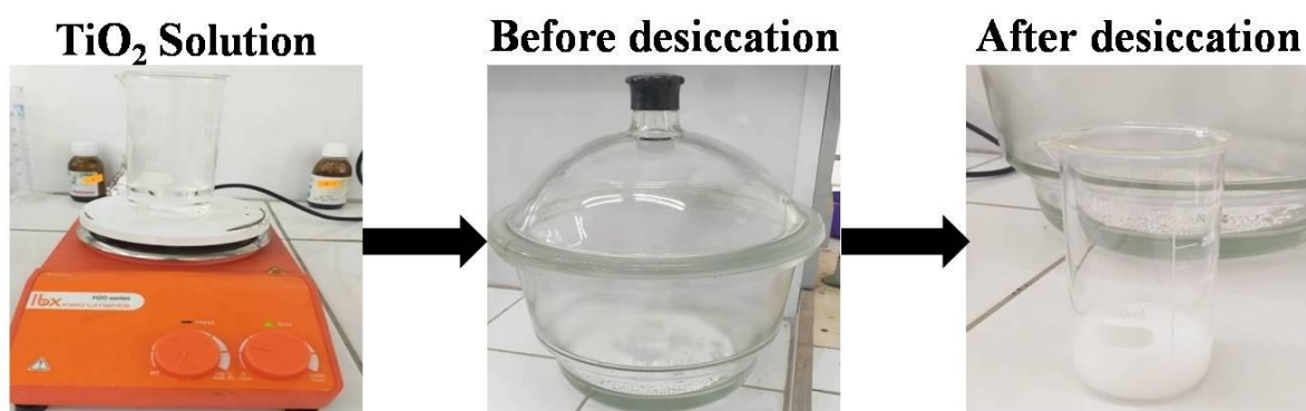
Figure 3. TiO 2 preparation procedure.
