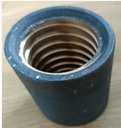
**Figure 9.** Bimetallic steel-bronze bearing.
